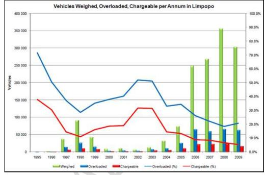
Figure 7-34: The Number of Heavy Vehicle Overloading Offences per Annum Charged at TCC's
